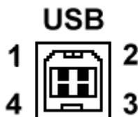
Figure 3-3: USB Connector pin orientation.
